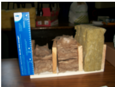
Goodworth Clatford Launch Showing correct loft insulation depth
